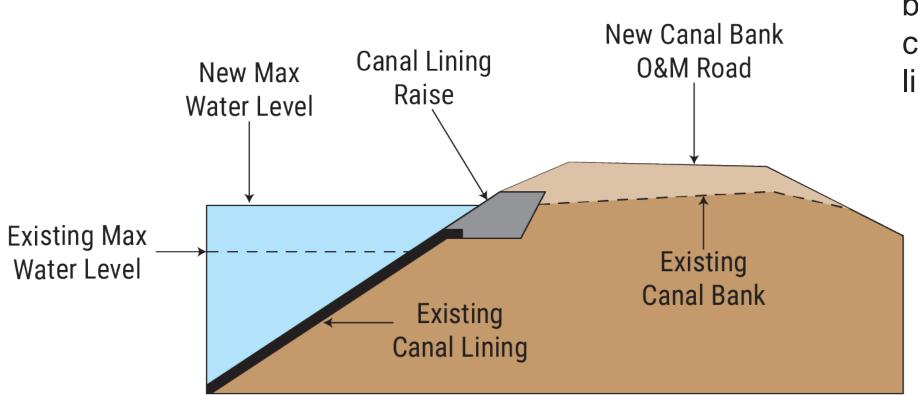
Segments 1 & 4 would be enlarged with a canal embankment and lining raise
