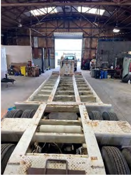
Lindsay maintenance staff removed and replaced damaged deck boards.
